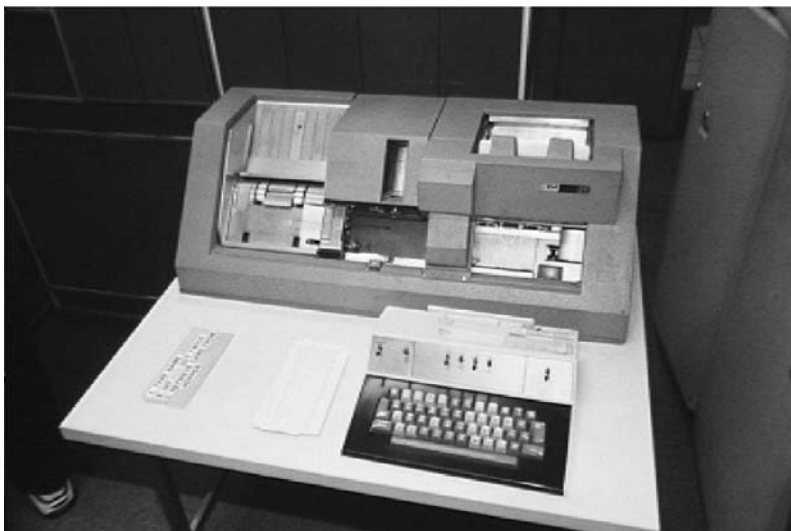
Fig. 1.8. An IBM Key Punch machine of the 1970s which operates like a typewriter except it produces punched cards (lying on the table) rather than a printed sheet of paper. Photo courtesy of IBM
