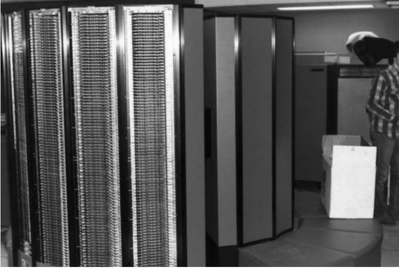
Fig. 1.9. The Cray X-MP, the world’s fastest supercomputer from 1983-1985 with a total operating performance of 800 Megaflops (Floating point operations per second). Note the Cray-typical circular arrangement of processor stacks. Photo courtesy of Michael John Muuss
